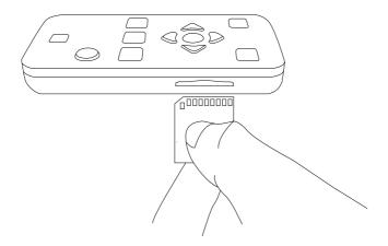
To remove the SD card, gently press the SD card into the card slot until it clicks, then release it. The SD card will pop out of the slot enough for you to grip it and pull it out completely. If the Blaze EZ is turned on, you will hear a sound to confirm that it has detected the removal of the SD card.
