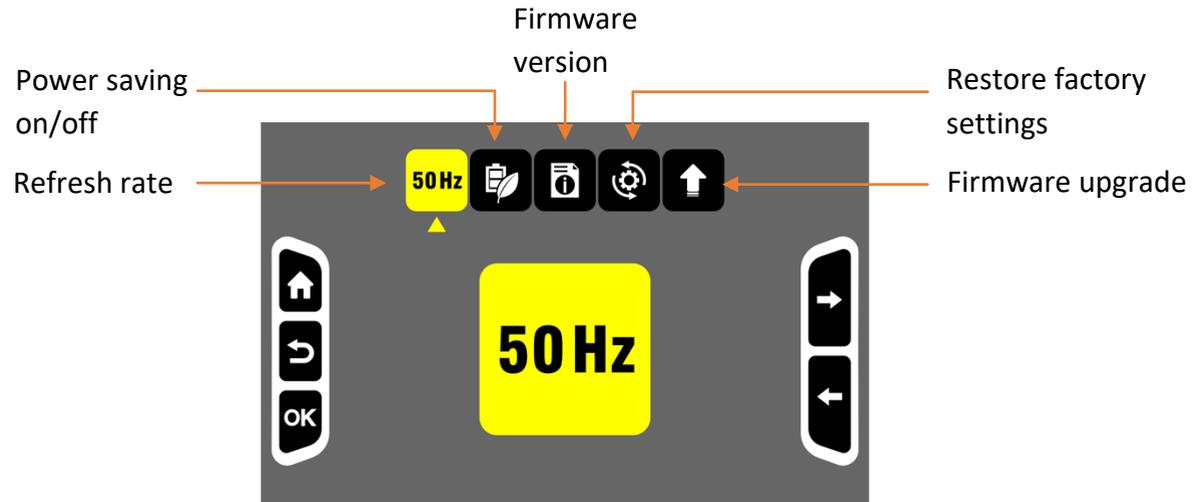
After entering the System Settings page, press Zoom in or Zoom out buttons to select the icon, press Mode button to confirm and enter the next level.
