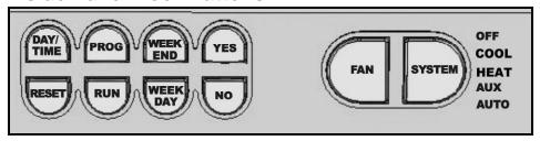
Most of the set up buttons are located inside the front panel door. Gently pull the door down to access the following buttons:
