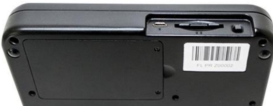
The battery compartment is located at the bottom of the device.
