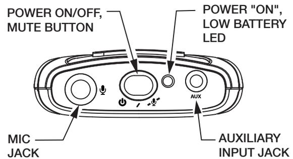
2. Plug the microphone cord into the “Mic Jack” (🎤) on top of the transmitter. (See Figure 2).
