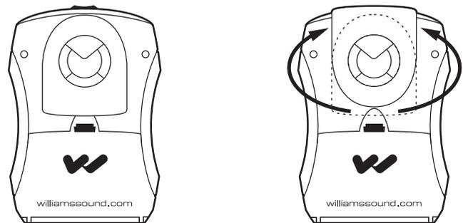
5. Install the belt clip on the rear of the T46 by positioning the belt clip on the back of transmitter. Turn the belt clip 180° left or right to secure the clip. The transmitter can now be clipped onto a belt. To remove, turn the belt clip 180° so the open end of the clip points up, and gently pull the belt clip off (See Figure 4).
